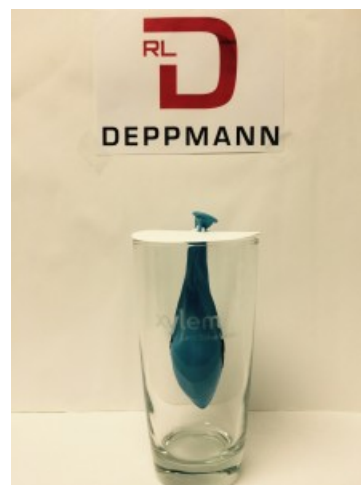
3 gallons of water have left the tank and the air side pressure is at its minimum of 78 PSIG
