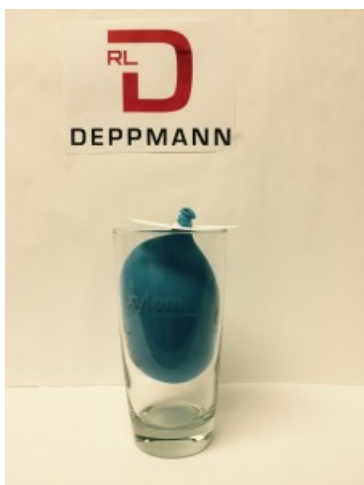
Tank is at maximum pressure and water is in the balloon. Example: 83 PSIG
